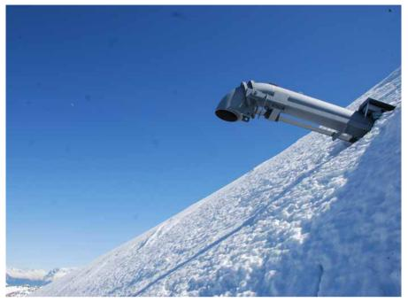
Figure 13: The effectiveness of new technology in risk management (here: GAZ-EX © avalanche release system) requires reliable and approved methodology for support of decisions by responsible experts
