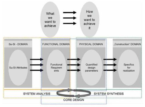
Figure 3: Conceptual planning steps – mappings in the design process (adapted from Suh, 2001)
