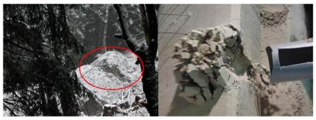
Figure 28 left: documented impact in embankment with failure. right: model test with similar behaviour
