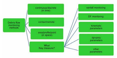
Figure 24: A proposed classification of debris-flow monitoring methods (adopted from Maček et al., 2014).
