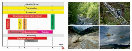
Figure 15: System of debris flow monitoring and warning technology, examples (Hübl & Mikoš, 2014)
