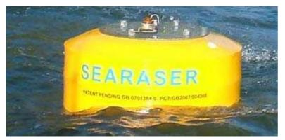
Pumping is made possible by the motion of waves lifting the device as it floats in the sea
